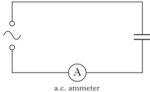
The a.c. supply has a constant peak voltage but its frequency can be varied.
