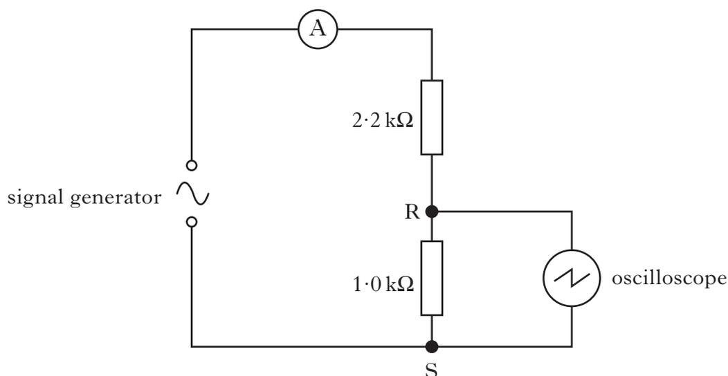
(a) An oscilloscope is connected across the  $1.0\text{ k}\Omega$  resistor.
