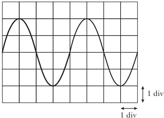
The timebase of the oscilloscope is set at 30 ms/div.
