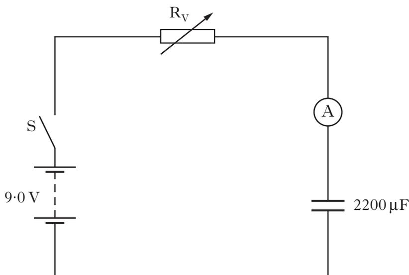
The battery has an e.m.f. of 9.0 V and negligible internal resistance.
