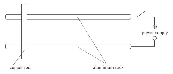
The apparatus is placed in a magnetic field. When the switch is closed, the copper rod rolls along the aluminium rods.
